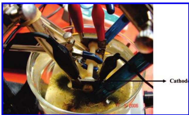
Figure 5. Generation of sludge around the cathode of the EC reactor.
